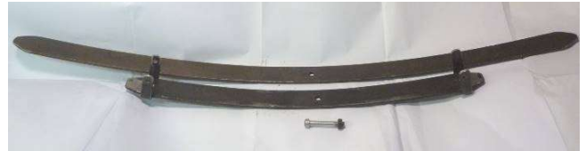
Cut down additional spring, existing lower spring with longer clips and extended central clamp peg
