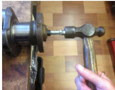
Pic 12: Removing the crank spigot bearing using the 'hydraulic' method
