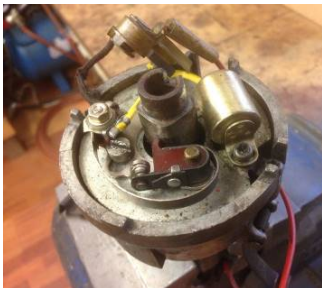
Pic 16: The original Lucas distributor set up with points and a condenser - quite complicated in a difficult to access area below the carbs.
