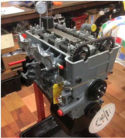
Pic 15: Cam timing using a dial gauge and circular protractor
