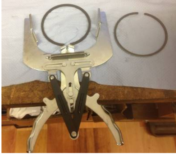
Pic 8: Piston ring assembly tool. Fitting rings, after checking the gaps in the bore, is always a bit tricky and I'm always nervous about breaking one. I find this tool, although a tad fiddly, helps greatly
