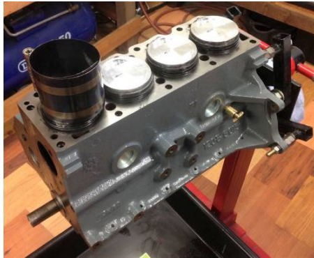
Pic 9: Pistons inserted in the block using a regular ring compressor. Watch the sharp edges!
