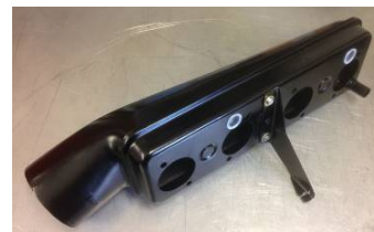
Pic 22: Correct Elan twin cam filter over a set of intake trumpets which has a conical K&N fitted on final assembly
