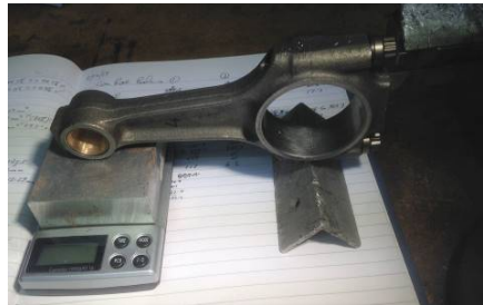
Pic 13: Checking conrod balance end to end using digital scales. Accurate measurements were taken with this set up on a surface plate.
