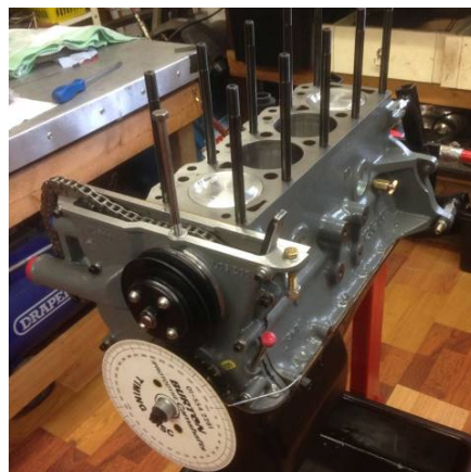
Pic 14: Engine block fitted with studs. The block threads are well cleaned and these studs are hand tightened to a 'nip', not torqued down.
