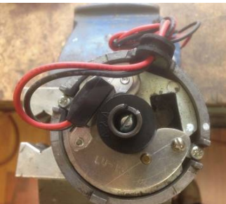
Pic 17: The upgraded distributor with much simpler and reliable electronic internals doing away with the points and condenser
